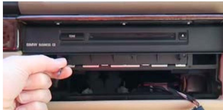
8. After that, you can pull out the CD player and unplug all the cable connected to the backside of player
