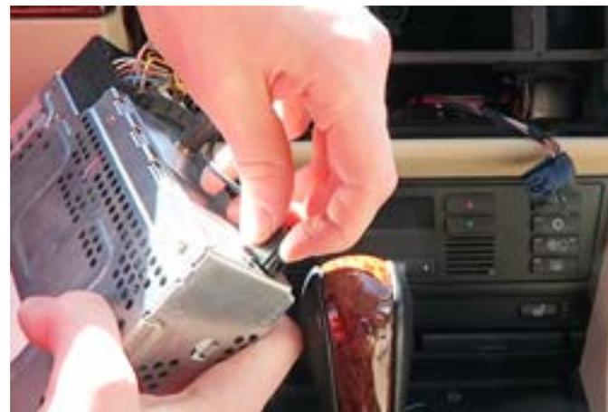
Now you can take out the power cable to connect the head unit and then try to turn it on. If this part is no problem, you can do the remain steps.
