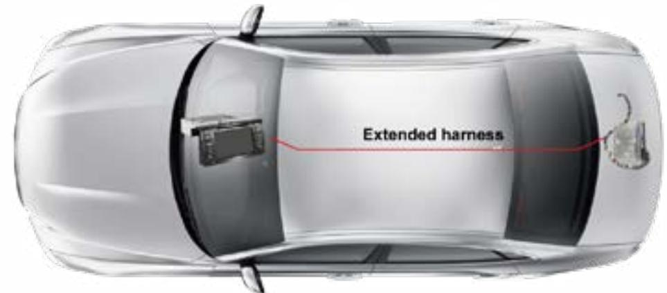
3. Connect the female radio plug of your car with the male plug of extended harness.
