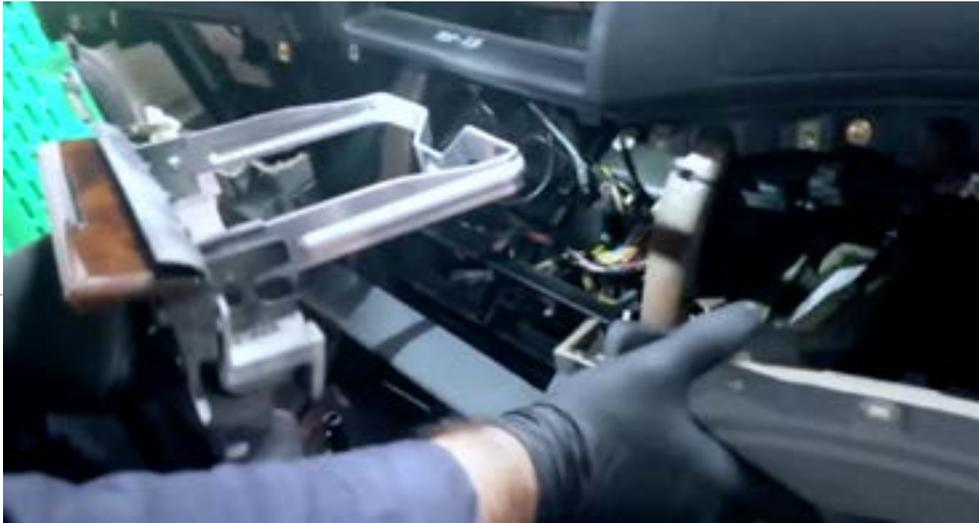
13. Screw back the bolts and then install the new bracket(12) to the both side of console.
