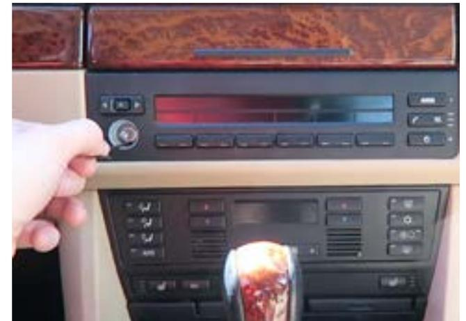
4. Turn the Allen wrench left and then you can pull out the whole radio.
