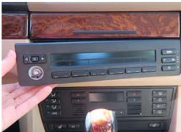
5. Moreover, unplug the cable connected behind the radio.
