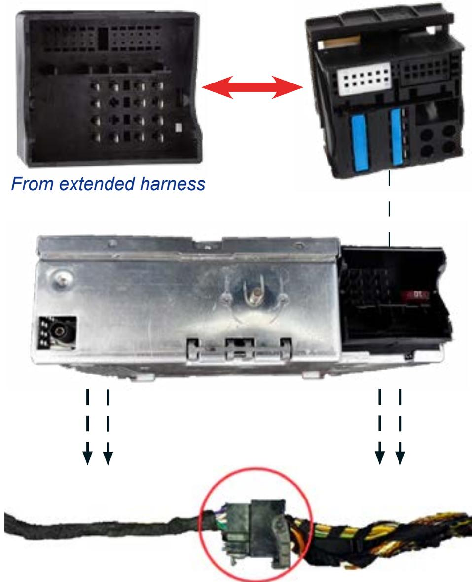
4. Connect the female plug of extension harness with the amplifier - BM54 tuner.
